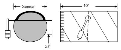
**Damper Specifications**Construction – 22 Gauge Galvanized Steel
